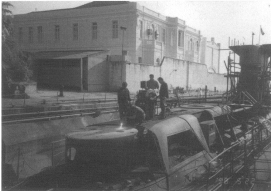
Fig. 3 Aluminum being sprayed on a submarine for the Brazilian Navy
